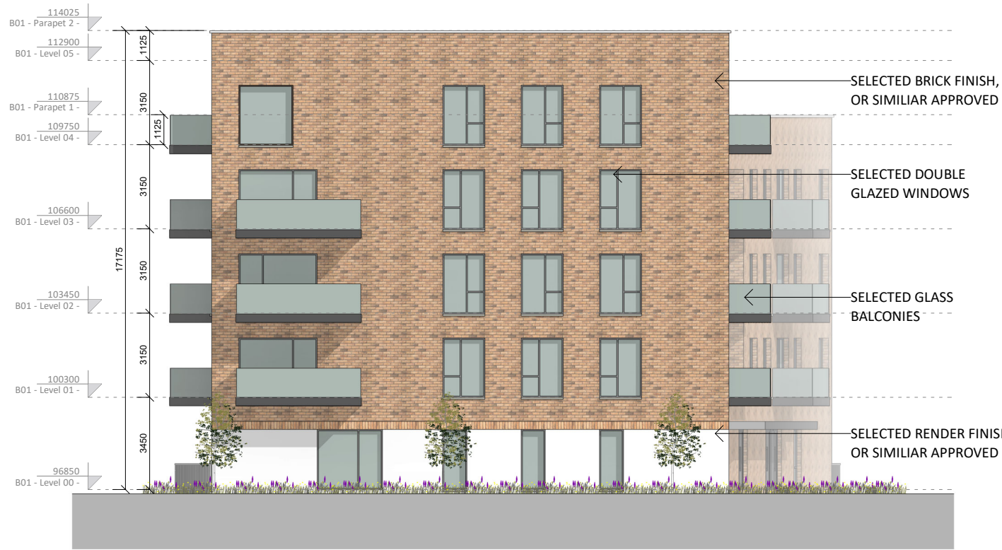
① Block 01 - North Elevation 1 : 200
